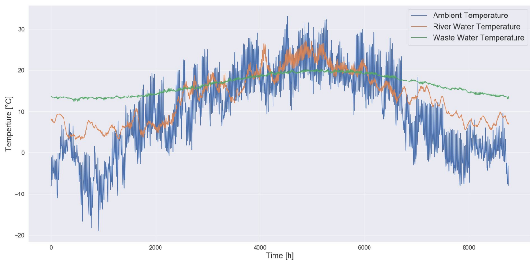
Figure 21: Temperature profiles for ambient air, river water and the outlet of the wastewater treatment plant used in the dispatch model (Source:(GDB, 2020), (ECO.S, 2018), (EU PVSEC, 2017))
