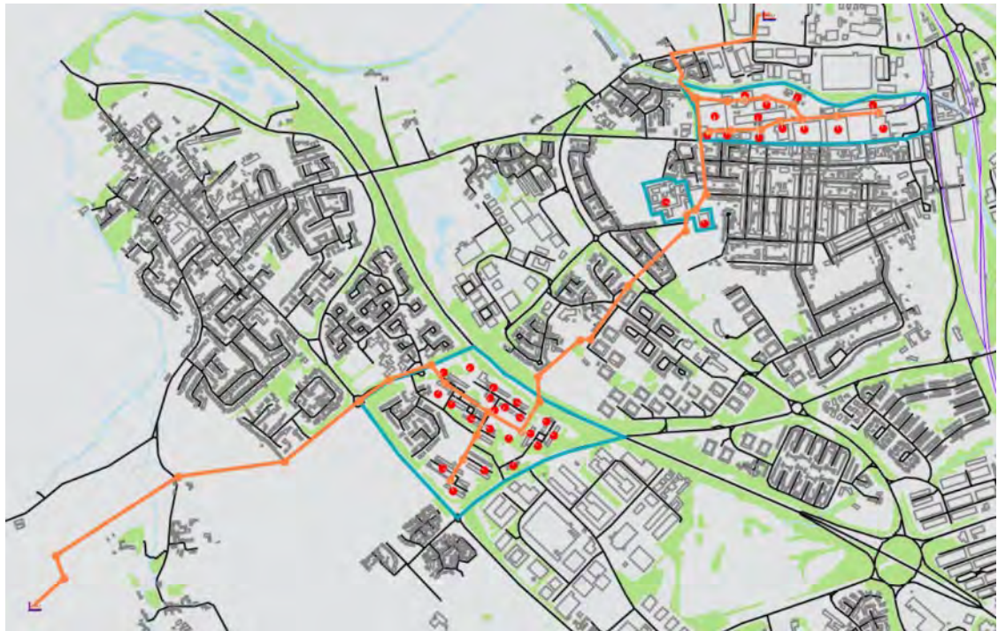
Figure 32 Potential district heating network path to supply buildings in Fullers Slade and Old Wolverton (DH design in Termis).
