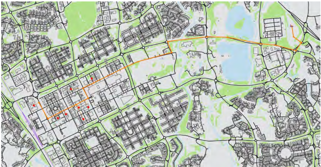
Figure 30 Potential district heating network path to supply buildings in Central Milton Keynes (DH design in Termis).
